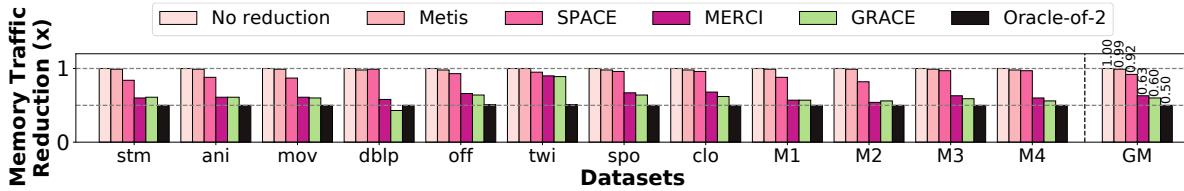
Figure 10: Memory traffic reduction in DLRM inference of compared works (lower is better).
