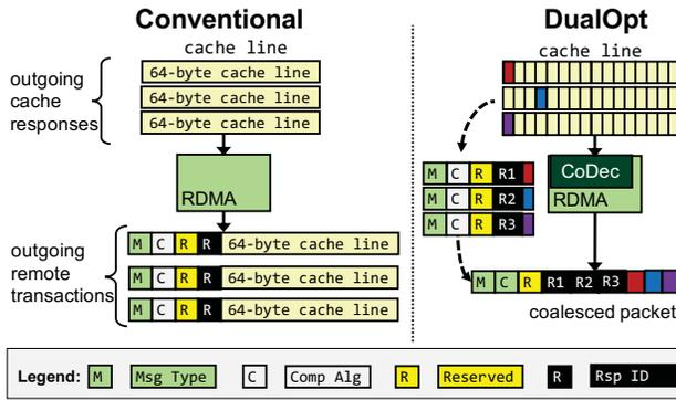
**Figure 9: Comparison of RDMA operations with and without CoDec.** A packet header includes the message type, compression algorithm, response ID, and few reserved bits. Packet sent to the same destination GPU carry similar header except the response ID. DUALOPT carries the response ID of each coalesced access for identification at the receiver.
