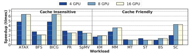
**Figure 18: Performance of DUALOPT with 4, 8, and 16 GPUs normalized to Baseline with 4, 8, and 16 GPUs.**
