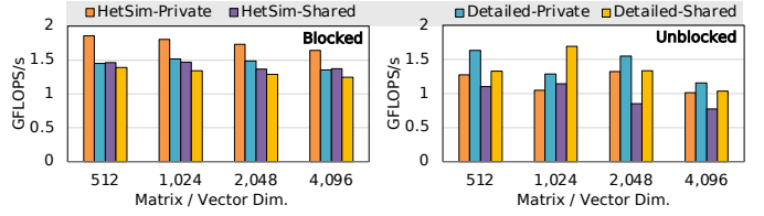
Fig. 11. Strong scaling performance comparison between different 4 \times 16 Transmuter configurations on two GeMV implementations, using HETSIM and the detailed model.
