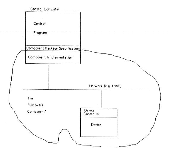
Figure 2: Software Component requiring distributed execution.
