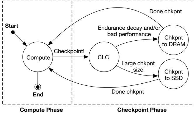
Figure 4.4: This state machine representing application execution shows how in the checkpoint phase the CLC dynamically decides the checkpoint location on each iteration.
