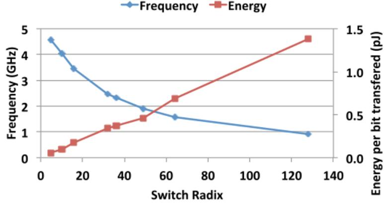
Figure 3.3: Scaling of a 128-bit Swizzle-Switch with radix.
