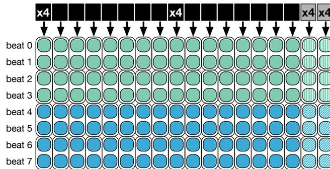
Figure 4.5: The depicted **normal ECC** access reads 512 bits from eighteen x4 chips, two of which are ECC chips. Two beats are paired up to create 1 8-bit symbol per chip. The first 4 and last 4 beats form two RS(36,32) codewords (green and blue).
