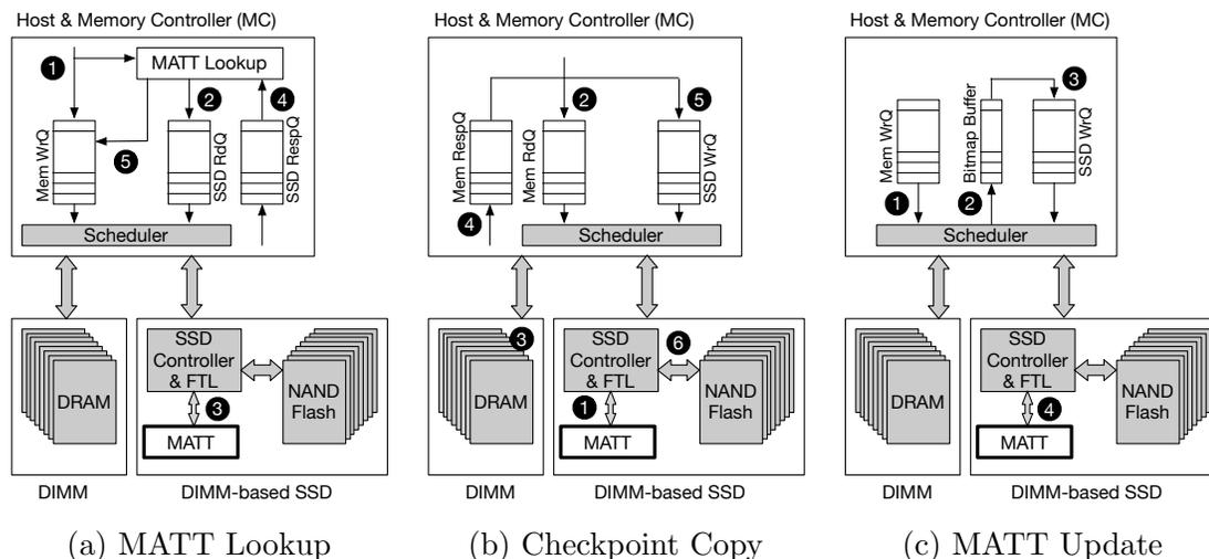
Figure 5.11: DIMM-based SSD with a MATT. (a) Write requests to DRAM look up the MATT to ensure that it’s not about to overwrite an uncheckpointed page. (b) The SSD Controller scans the MATT and initiates checkpointing. (c) The block number of each write request is saved to the bitmap buffer as it’s processed by the memory controller.
