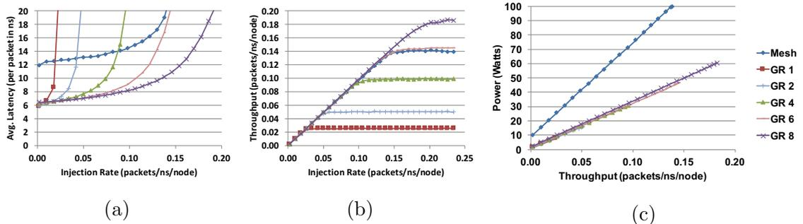
Figure 3.14: Energy proportionality of Super-Star topology with varying number of global routers:(a) Network latency (b) Network throughput and (c) Network power.
