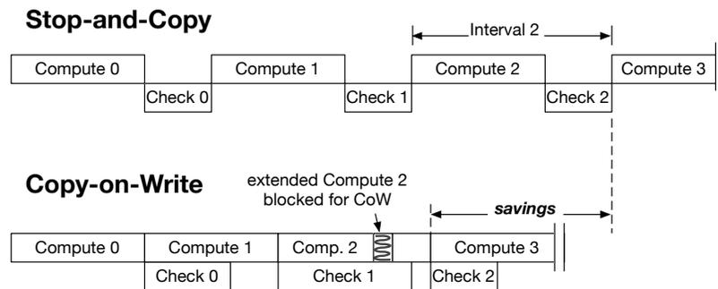
Figure 5.1: Timing overheads by conventional checkpointing methods
