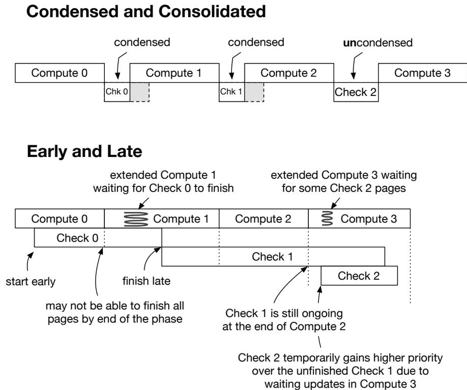
Figure 5.10: Timing overheads by the new checkpointing methods
