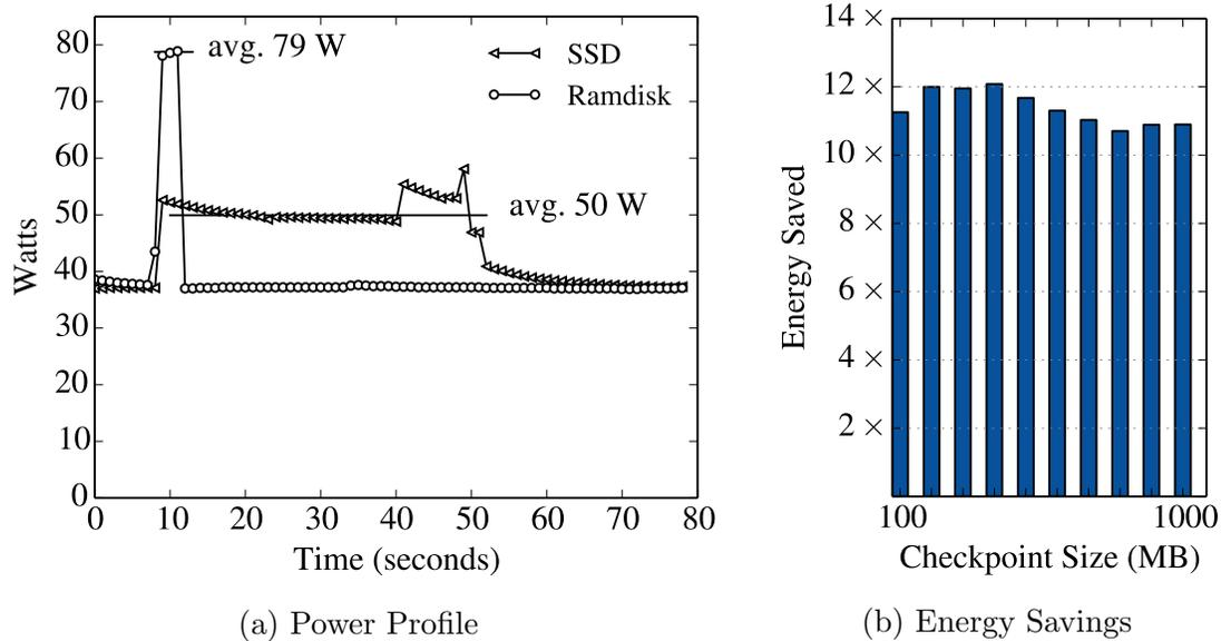
Figure 4.12: (a) The SSD consumes 50W during a write operation, whereas the DRAM consumes 79W. (b) However, due to DRAM’s faster write bandwidth, redirecting some checkpoints to the DRAM saves overall checkpoint energy.
