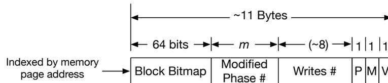
Figure 5.9: A Memory Accesses Tracking Table (MATT). *P*=this page is top *priority* for checkpointing because a write request is blocked and waiting, *M*=this page was *modified* again after it was checkpointed early, *V*=this page is *valid* in memory.
