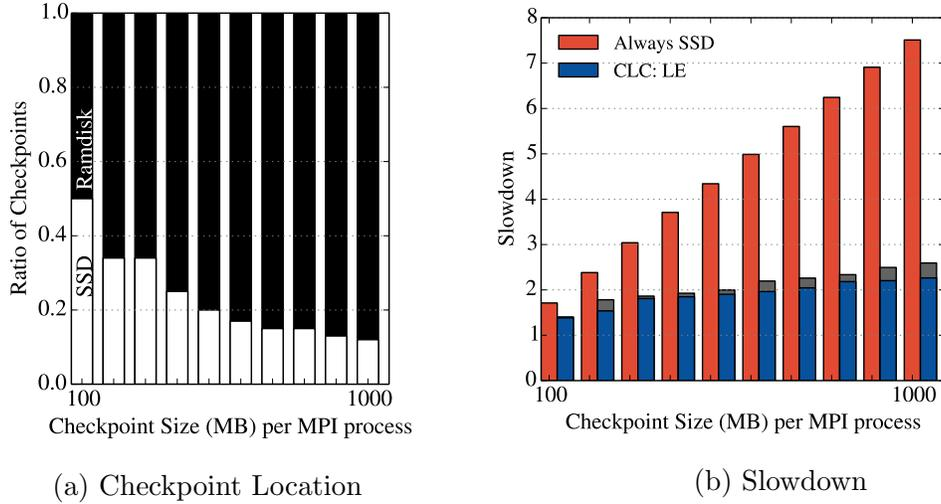
Figure 4.8: Microbenchmark results with the CLC’s lifetime estimation (LE) feature enabled. (a) For bigger checkpoint sizes, more checkpoints are written to the ramdisk. (b) The CLC significantly reduced the slowdown. The shaded region above each bar is the overhead for strong ECC’s second memory access.
