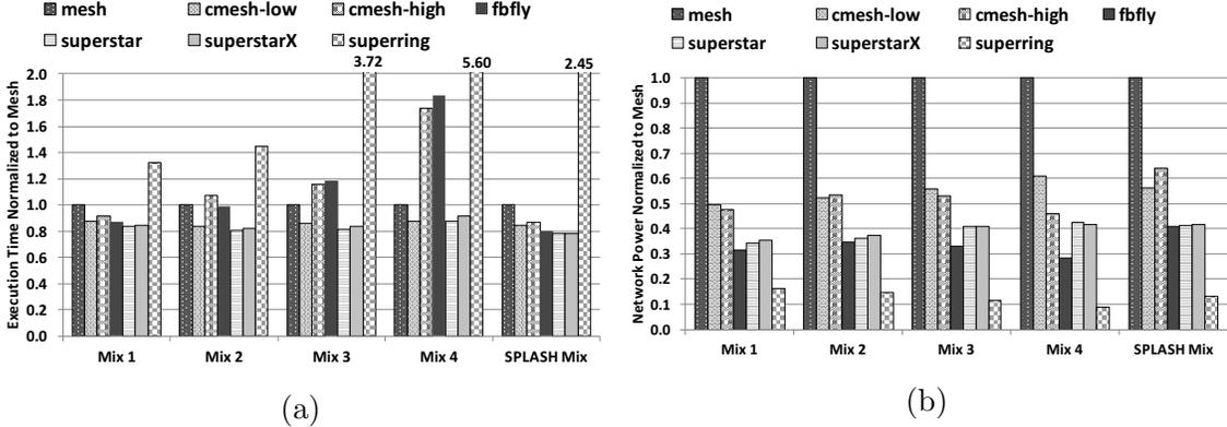
Figure 3.16: Performance of different topologies with application workloads: (a) Execution Time (a) and Network Power (b)
