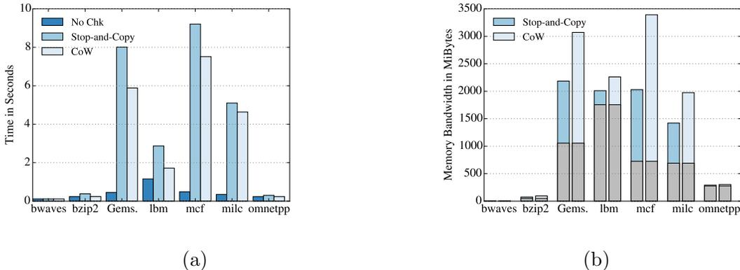
Figure 5.2: Checkpoint results (a) runtime and (b) memory bandwidth with conventional *stop-and-copy* and *copy-on-write* methods. Although *copy-on-write* improves performance, it is at the cost of extra memory bandwidth use.
