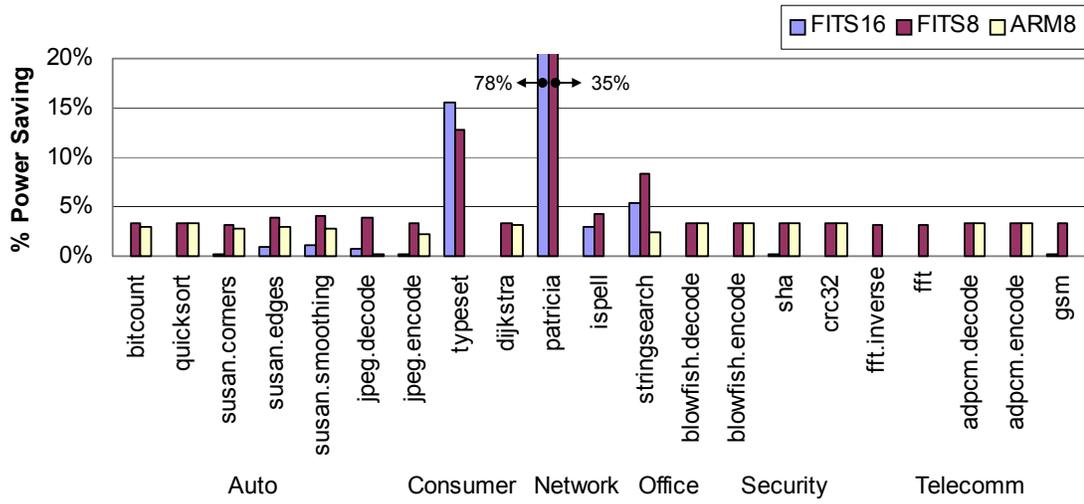
**Figure C.3: Chip-wide Leakage Power Saving**
