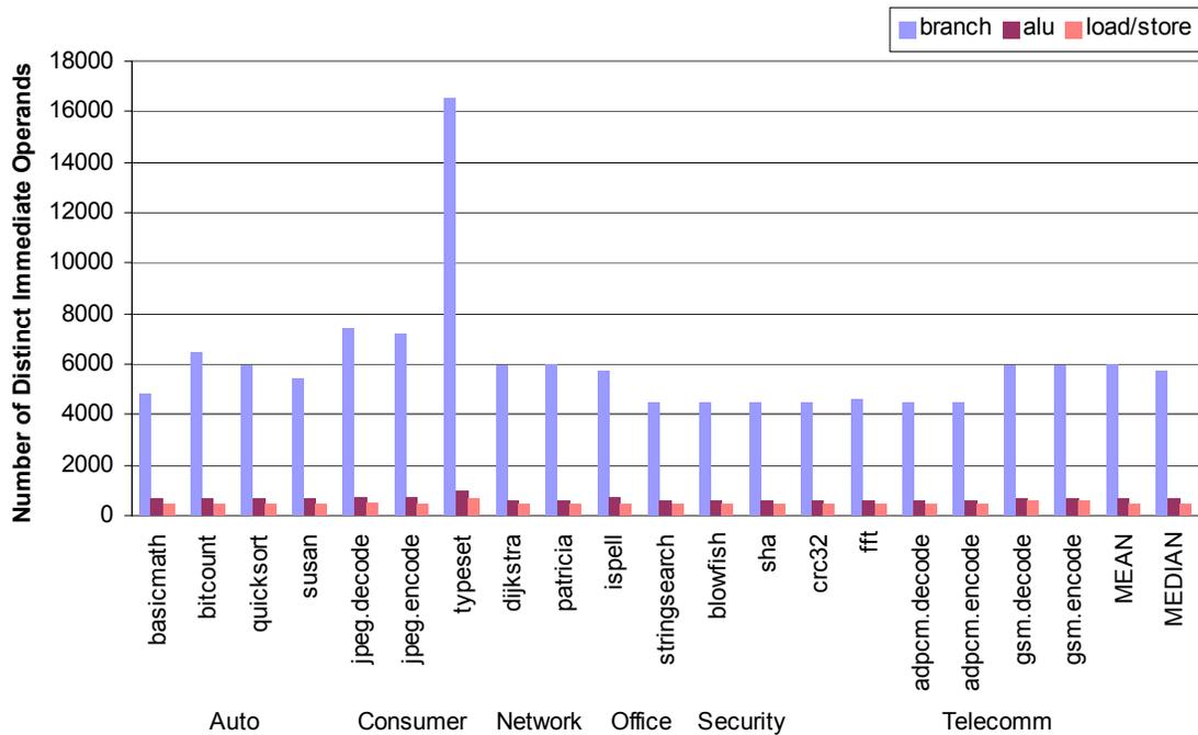
**Figure 2.6: Static Utilization of Distinct Immediate Operands**
