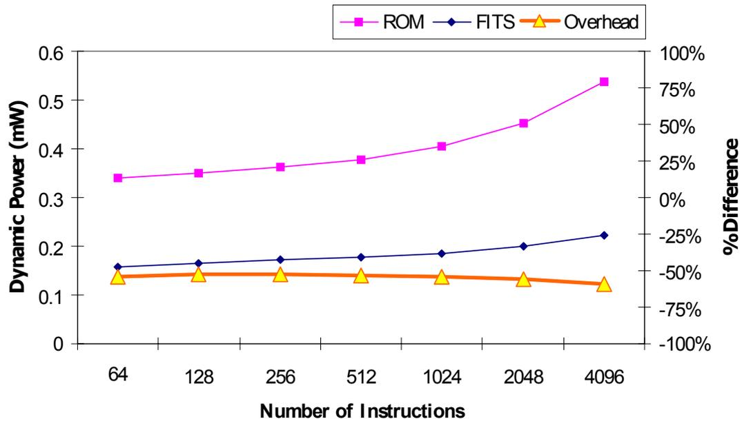
**Figure 5.4: Dynamic Power Comparison between Fixed and FITS Decoders**
