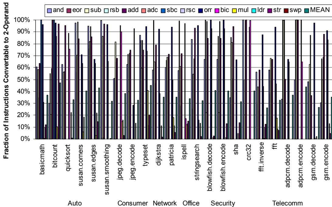
**Figure 2.4: 2-Address Compatible Dynamic Instruction Distribution**
