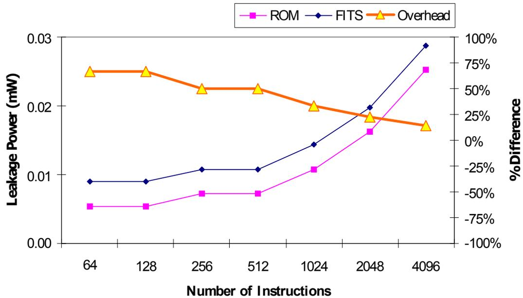
**Figure 5.3: Leakage Power Comparison between Fixed and FITS Decoders**
