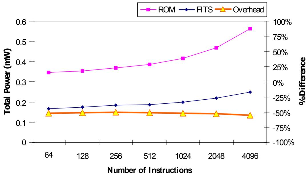
**Figure 5.5: Total Power Comparison between Fixed and FITS Decoders**
