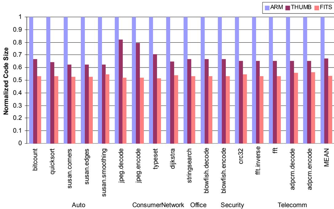
**Figure 5.8: Code Size Comparison between ARM, THUMB, and FITS**
