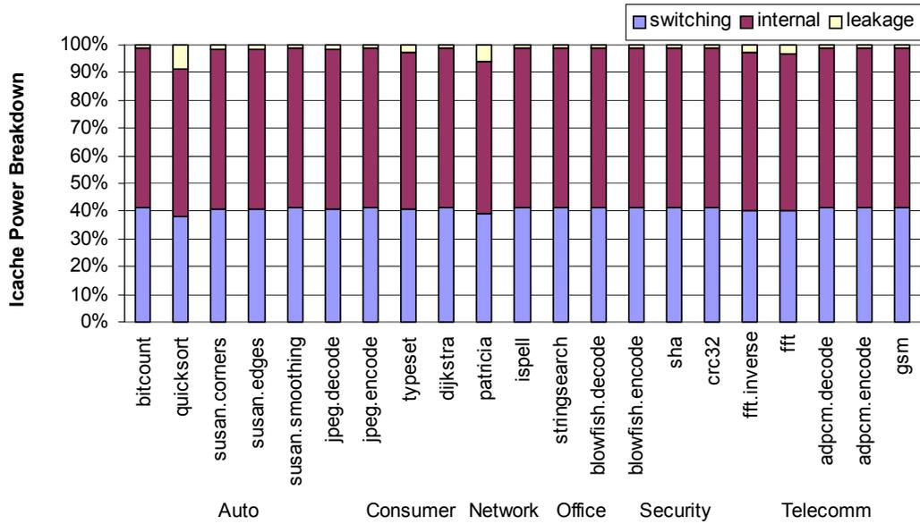
Figure A.1: Instruction Cache Power Breakdown for ARM8
