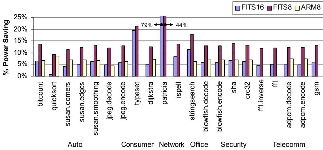
Figure C.1: Chip-wide Switching Power Saving
