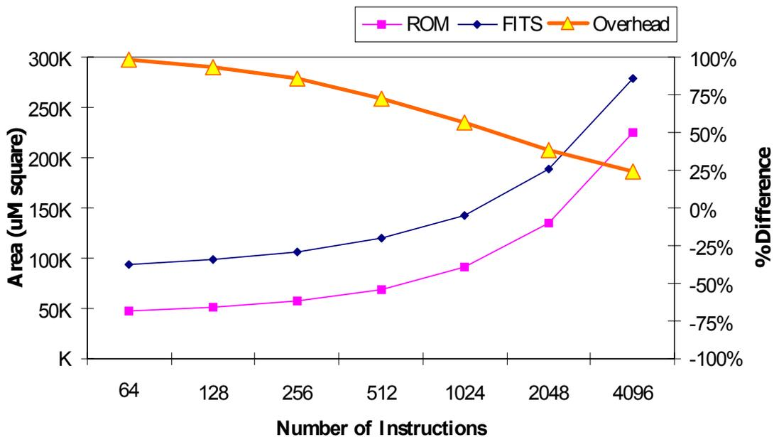
**Figure 5.1: Area Comparison between Fixed and FITS Decoders**
