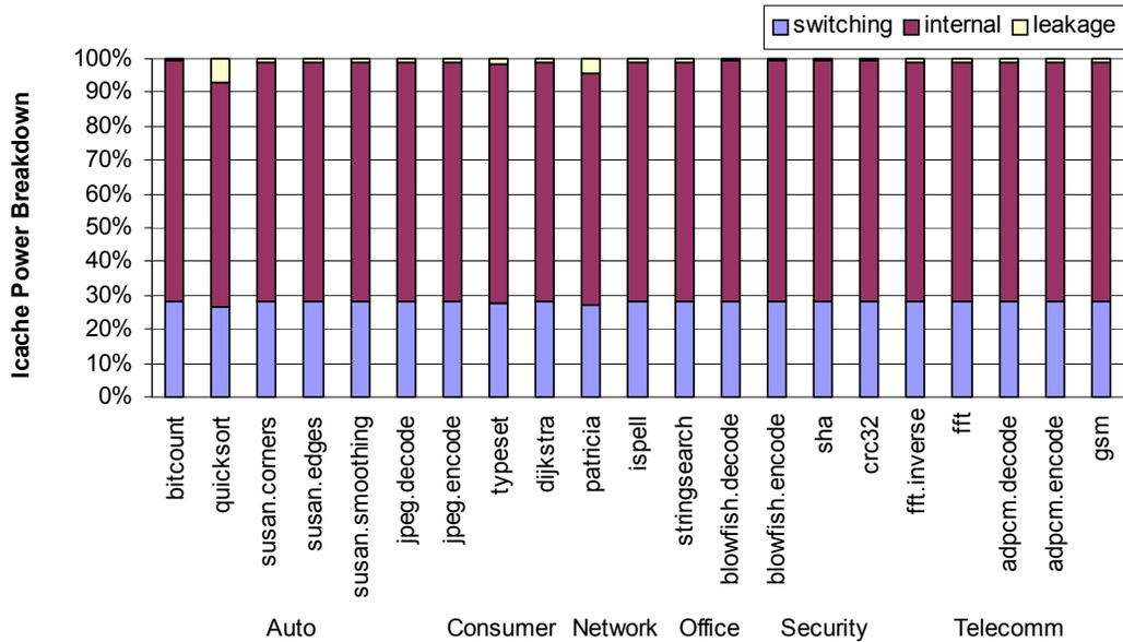
Figure A.2: Instruction Cache Power Breakdown for ARM16
