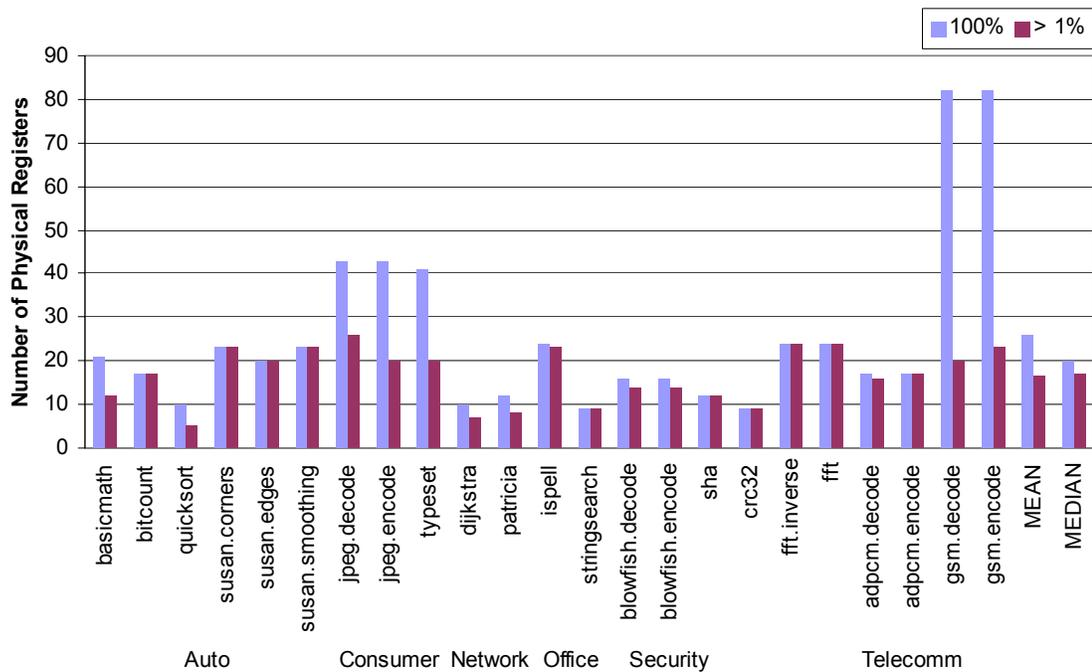
**Figure 2.9: Utilization of Physical Registers**
