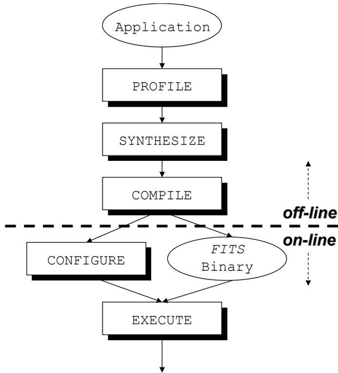
**Figure 3.1: System Design Flow of FITS Framework**
