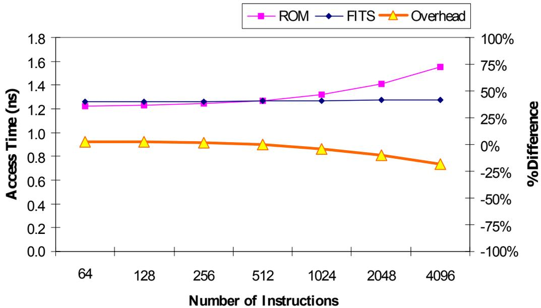
**Figure 5.2: Access Time Comparison between Fixed and FITS Decoders**
