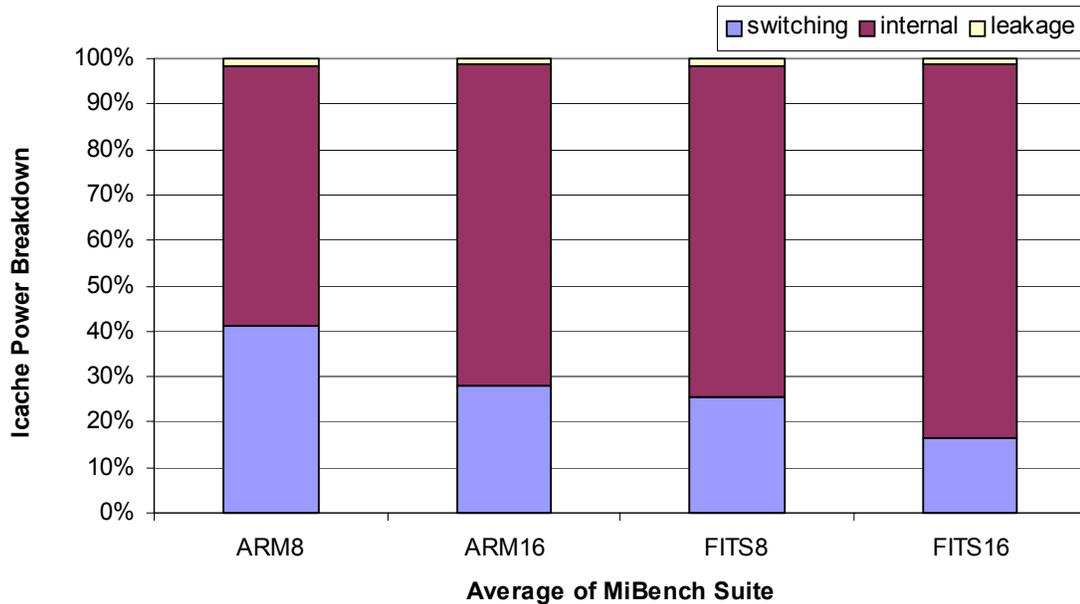
**Figure 5.9: Instruction Cache Power Breakdown for ARM and FITS**
