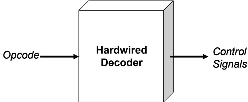
**Figure 3.13: Conventional Hardwired Instruction Decoder**
