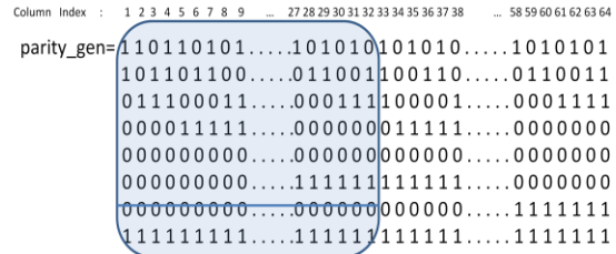
Figure 9. Parity generation for (39, 32) from (72, 64).
